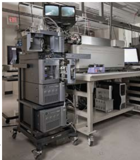
YCCI funded the purchase of the Waters nanoACQUITY UPLC® System, which provides high resolution chromatography for protein identification and characterization.
